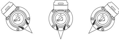
**Fig. 2** Terminal box positions, single-head pumps
